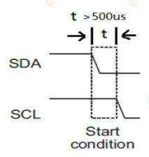
Note: This module can be wakeup by I2C interface. There are some limitations when the module is wakeup by I2C interface. For the first "start" command of the I2C protocol, the SCL will have to hold at least 500us to wake up MCU. The maximum I2C clock is 100 KHz.
